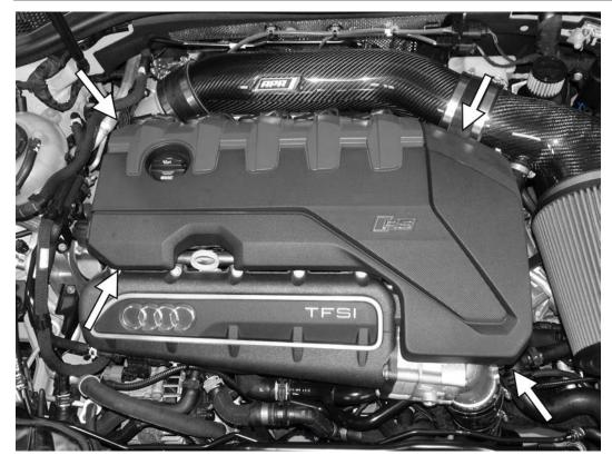
3) Remove the engine cover by carefully lifting each of the four corners, popping the cover off the mounting posts.
