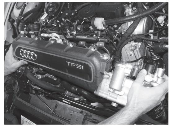
9) Carefully rotate the top of the upper portion of the intake manifold with throttle body attached away from the engine. Then lift to remove the assembly from the car.
