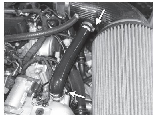
35) If the car has an APR intake, install the supplied hose between the DV outlet and the port on the APR intake. Secure the hose with the two supplied hose clamps.
