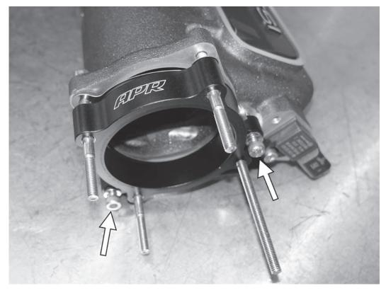
21) Install the APR spacer onto the three screws in the upper intake manifold as shown. Secure the spacer to the manifold with the two supplied 25mm screws with a flat washer on each screw. Torque these two screws to 9Nm (80 in-lbs).
