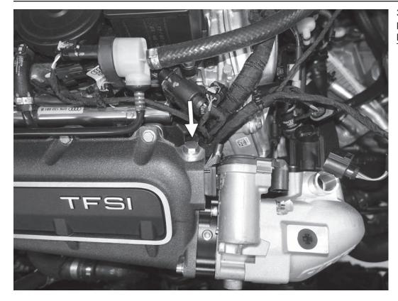
31) If installing the APR cast inlet pipe on a later car, install the supplied 13mm plug with crush washer. Torque the plug to 32Nm (24 ft-lbs).
