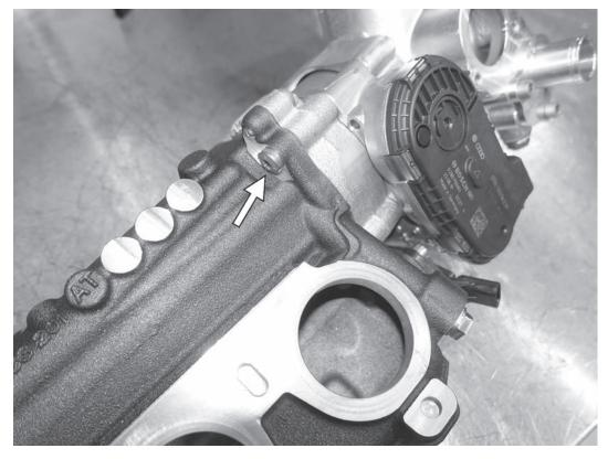
13) On the back side of the upper manifold assembly, remove the T30 screw holding the throttle body to the intake manifold.
