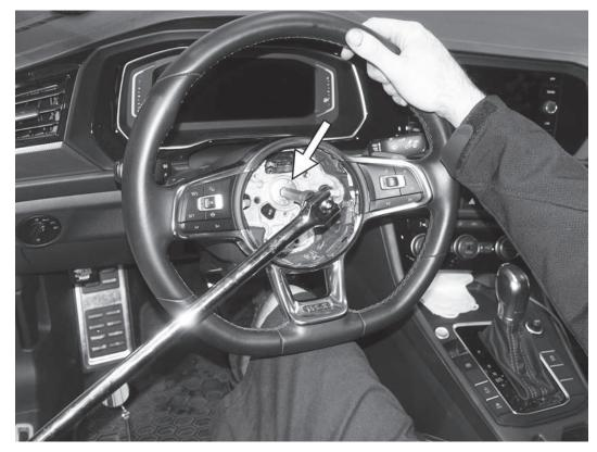
9) Using a 12mm triple square and a breaker bar, loosen and remove the bolt holding the steering wheel in place. Do not remove the steering wheel.
