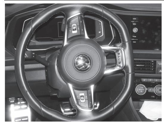
5) With one side of the airbag slightly popped off, turn the steering 180° the other way to access the other slot behind the right wheel spoke.
