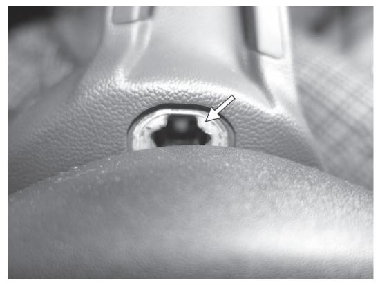
3) On the back side of the steering wheel, on the left wheel spoke facing up, locate the metal slot.
