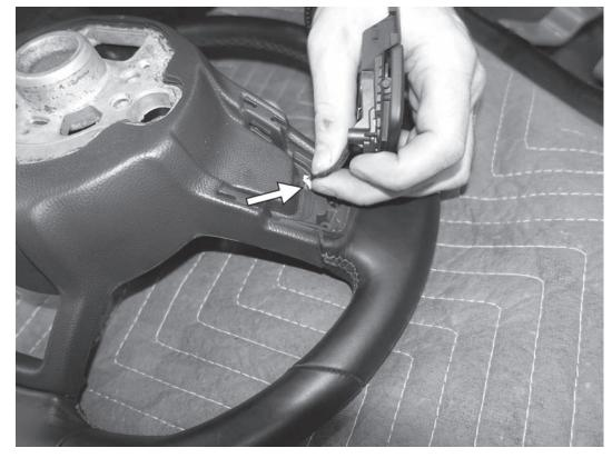
19) Remove the DSG paddles from the back of the steering wheel, and carefully pull the harness and connector through the steering wheel.
