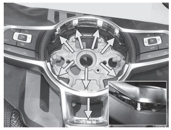
11) There are eight posts holding the plastic steering wheel trim to the steering wheel. The posts, shown in the inset picture, will all need to be separated in order to remove the trim. A fair amount of force is necessary, but be careful not to break them.
