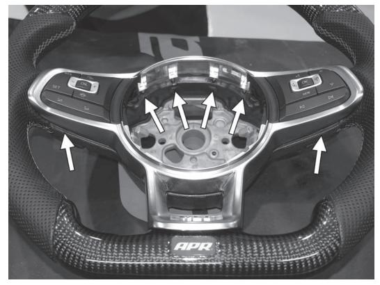
23) Work around the wheel from the bottom up, ensuring all the mounting posts are going into the correct mounting holes in the steering wheel.
