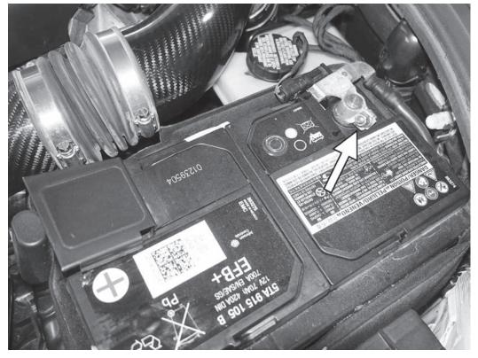
1) Disconnect the negative battery terminal by loosening the 10mm nut and lifting the battery cable off and away from the battery.
