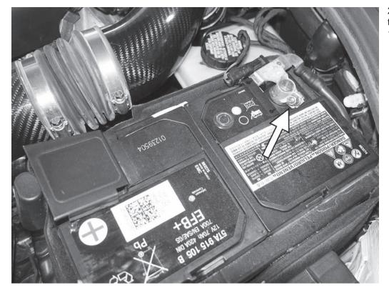
27) Reconnect the negative battery terminal to the car, and tighten the 10mm nut to 9Nm (80 in-lbs).
